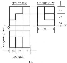
Q.5(B) Draw the Front view, Top View and Side view for the figure given
