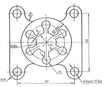
Draw the above figure using AutoCAD Commands
