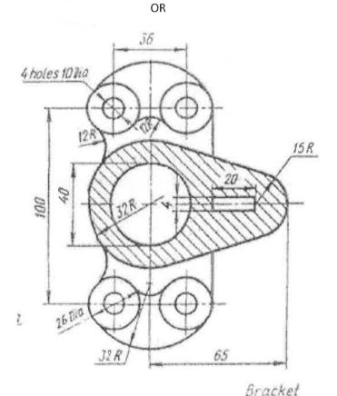
Draw the above figure using AutoCAD Commads
